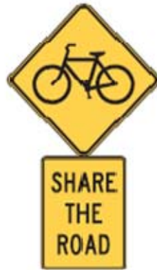
Figure 3.3 SHARE THE ROAD assembly W11-1 and W16-1
