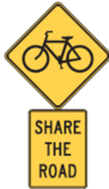
Figure 3.3 SHARE THE ROAD assembly W11-1 and W16-1
